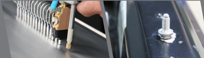
Weld special Alu-Bits for the repair of Aluminum Panels with VAS 6321
