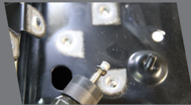
Weld special Alu-Bits for the repair of Aluminum Panels with VAS 6321
